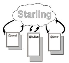
The general I/O pins of the Starling are defined as inputs on start-up and each pin has an internal pull-up. When an I/O pin is shorted to the ground, this fires a "input status changed" event and the <code>@input</code> function in your script will run.\* The <code>@input</code> func-
