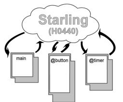
The general I/O pins of the Starling are defined as inputs on start-up and each pin has an internal pull-up. When an I/O pin is shorted to the ground, this fires a "input status changed" event and the @input function in your script will run.\* The @input function then handles the event, perhaps by
