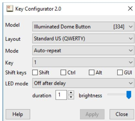
The utility configures only a single button at a time. The serial number, at the right of the model name, shows which button is being configured. The last
